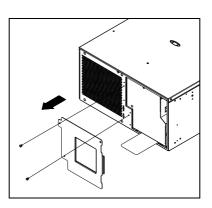
(2) Remove the retaining screws of the cable protection cover, and then remove the cover itself.
